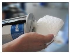
Adjust working pressure at the regulatin valve to 1,5 - 2 bar. Put on static mixing nozzle MFHX 06-32 in vertical position, fasten it and fill it with material right to the tip of the static mixing nozzle.
