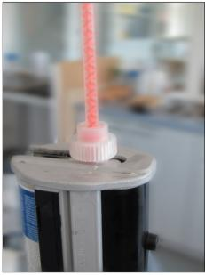
The sealing compound can now be extruded. During breaks and whenever the pistol is put down please always put a cloth under the tip of the mixer to collect excess material. Wipe static mixing nozzle tip clean before restarting work.
